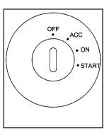
The ignition switch is located on the instrument panel, to the right of the steering column.
